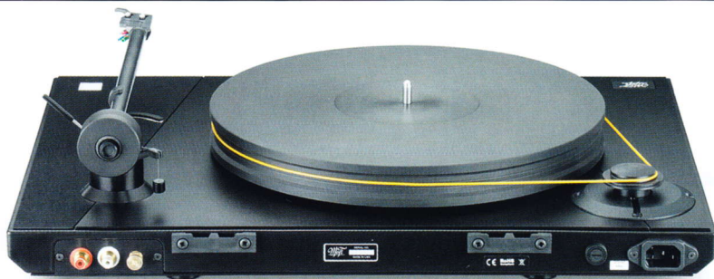
ABOVE: No external PSU here but (unusually) a direct AC mains power connection. Tonearm wiring is by Cardas Audio, terminated in RCA outputs and a ground post
